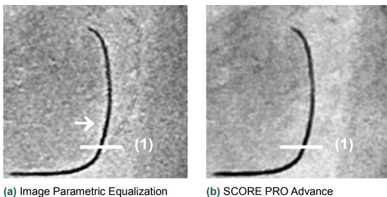
**Fig. 3** Example of Edge Enhancement
