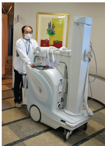
Fig. 2 MobileDaRt Evolution Incorporating a New, Thin, Large-Field-of-View FPD
