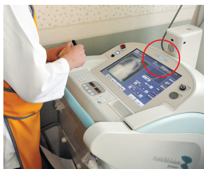
Fig. 7 Illuminated Indicators Colors indicate the Standby, Ready, or Exposure status.
