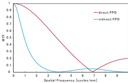
Fig. 3 Comparison of MTF Between Direct FPD and Indirect FPD
