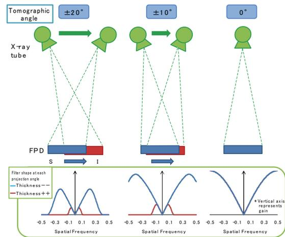
Fig. 4 Changes to Reconstruction Filter Shape at Each Projection Angle
